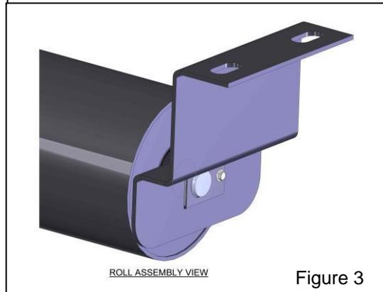
First, install both hanger brackets loosely into place below belt conveyor frame side stringer.
