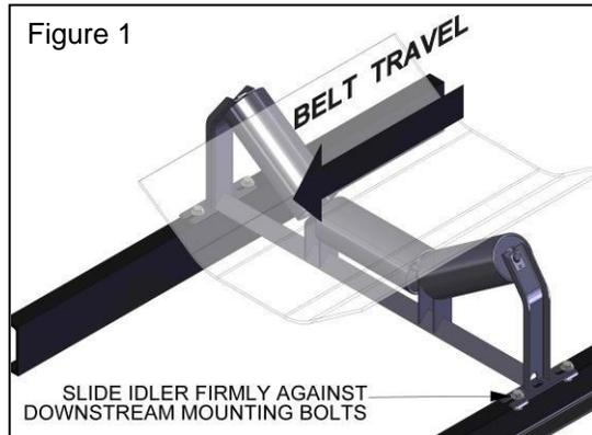
Place idlers in position by sliding them in the direction of belt travel until the foot brackets seat against the mounting bolts (see figure 1). Tighten all mounting bolts by hand. Final alignment requires that the centers of all idlers are in a straight line, perpendicular to the line of belt travel, properly spaced, and level. When alignment is complete, tighten all idler mounting bolts.
