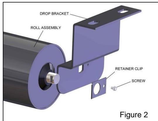
After the trough idlers have been set in place, the return idlers should be installed. The return idlers must be installed perpendicular to the conveyor centerline and level. Leave the training idlers out until the belt has been properly trained.
