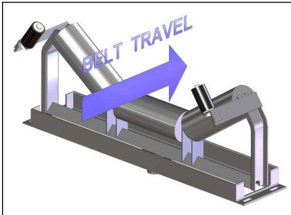
Self-aligning trough idlers are installed along the conveyor length, as required, but no closer than 50 feet from any pulley. Positive arm type units are used on belts traveling in one direction only. Actuating type trainers (without arms) are used on reversing belts and on belts with traveling trippers or stackers.
